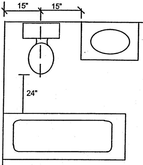
Figure 84.20-3. Spacing between water closet and tub.
